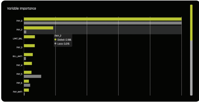
Global (yellow) and local, i.e. row-wise (grey), variable importance for a Driverless AI model.
